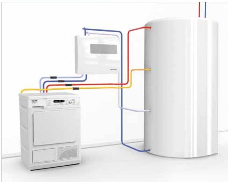
*The new solar dryer dries laundry using hot water from the solar thermal plant, and thus reduces costs by up to 80 percent.*
